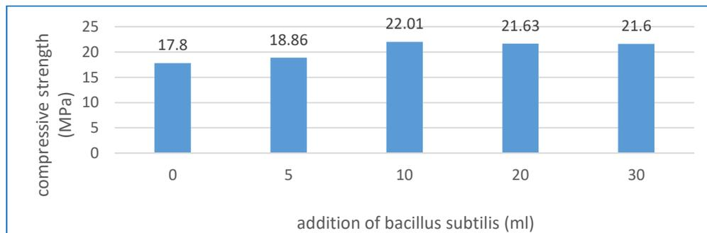
**Fig 1: Compressive strength for varying bacillus content at seven days**
