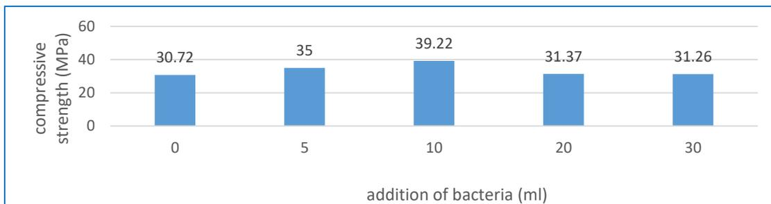
**Fig 3: Compressive strength for varying bacillus content at seven days**
