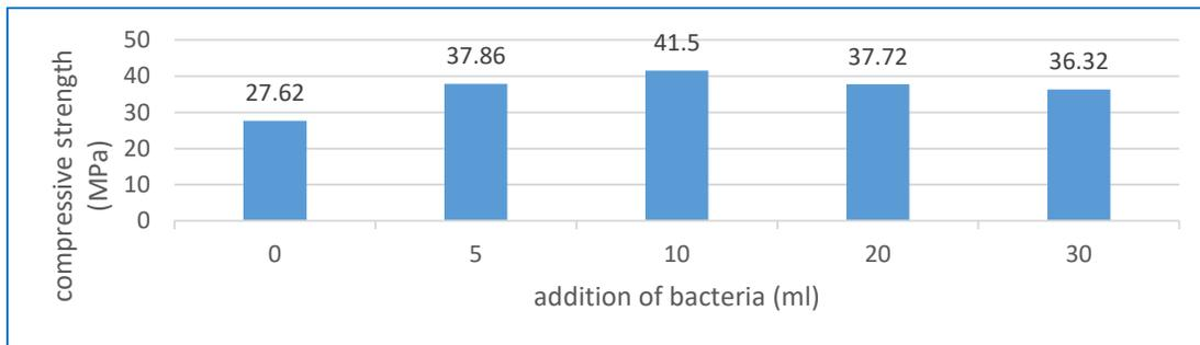
**Fig 2: Compressive strength for varying bacillus content at 28 days**
